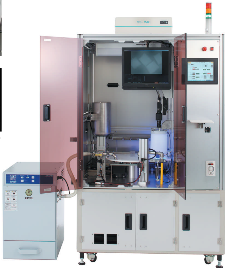
Detects foreign matter or discoloration among Pellet and Granule
